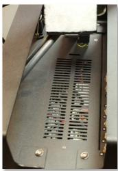
4. Use an air blow gun or a can of compressed air to remove debris from the filter.
