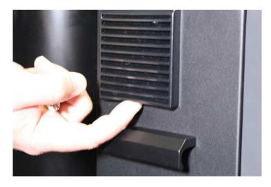
3. Lift up on the bottom of the housing to release the tab, then pull away to remove.
