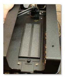
3. Loosen the captive screw and pull up on the air filter housing to remove.
