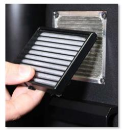
4. Use an air blow gun or a can of compressed air to remove debris from the filter.
